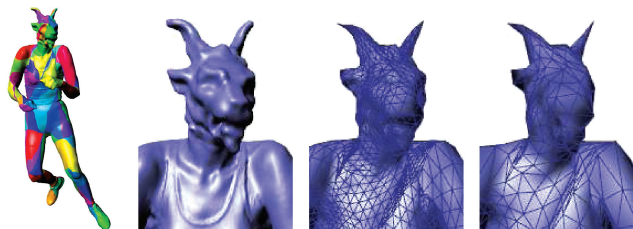
Fig. 13. Triangular charts and reconstructed meshes at varying levels of detail for a BOXING animation.
