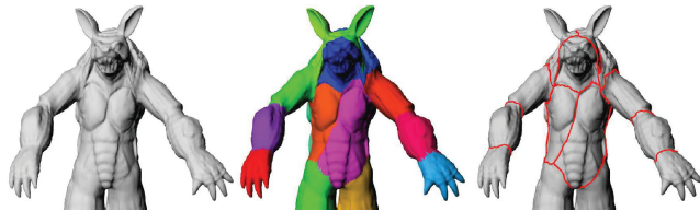
Fig. 6. Triangle clusters and their boundaries resulted from our new metric for spectral clustering using deformation gradients from the BALLET mesh animation.
